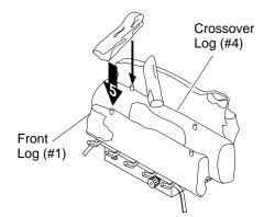
Figure 32 - Installing Crossover Log (#5) (CCL3018NT Only)
